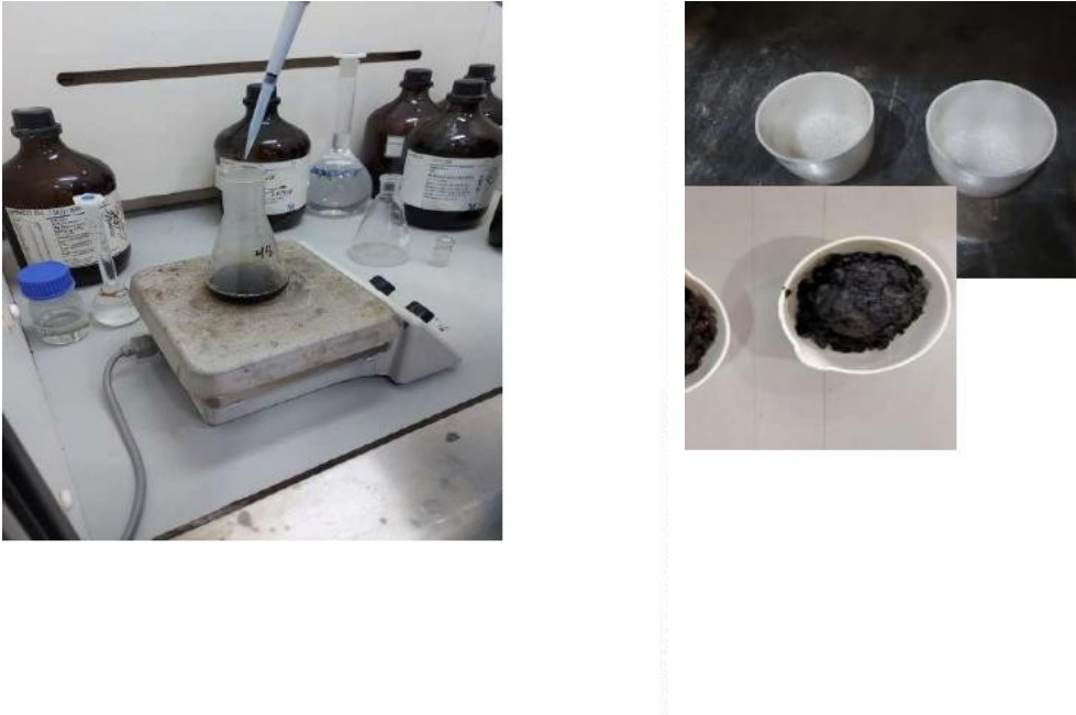
Figure 8: Laboratory measurements of Raincatcher chemical parameters (to the left, the acid digestions of Raincatcher and to the right, the determination of moisture and ash content)
