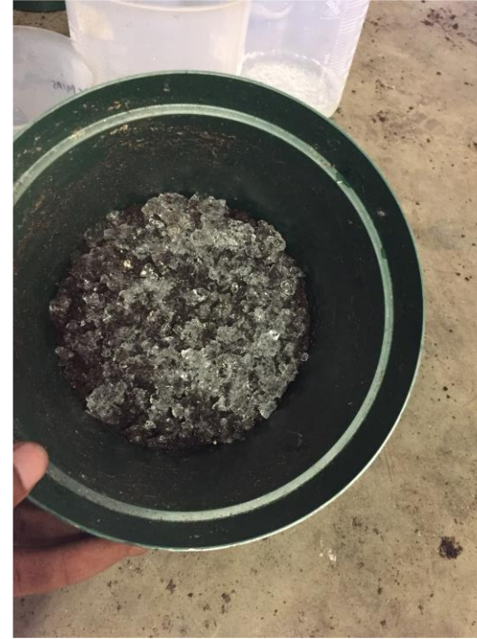
Polymer hydrated then added to soil
